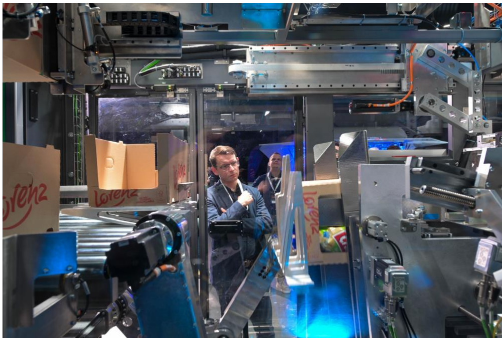
Caption: Focke and Lorenz: Joint Project “Phoenix Universe” – Compact Modules for Complete Secondary Packaging and Palletizing ©Lorenz Snack-World
